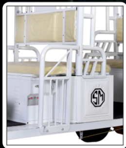
MIDDLE BOX WITH "SM-SPEEGO MORNI" DIE STAMP, 3 BATTERY & STEPNEY INSIDE
